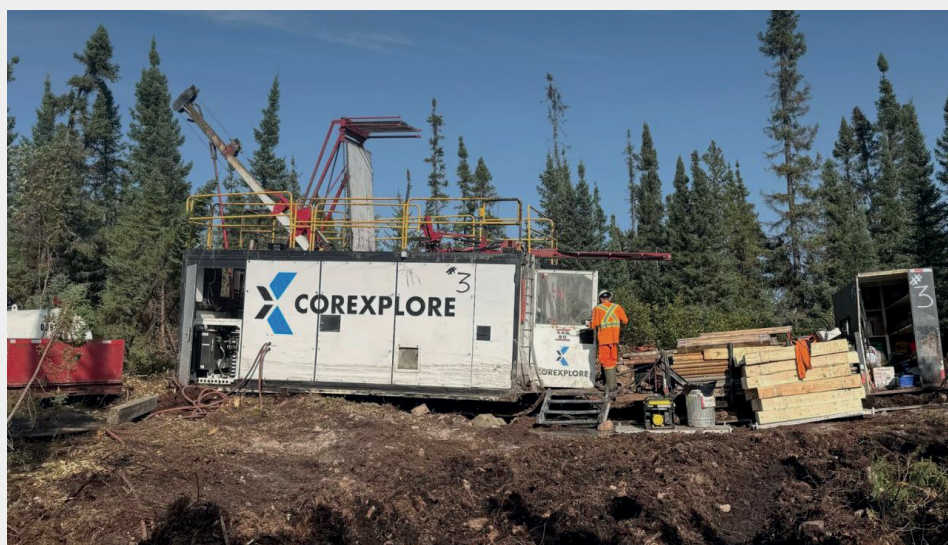
Boots on the ground at La Grande. A Corexplorer diamond drill rig turns in the boreal forest at Zone 32 during Lux's 2026 drill program, with stacks of core boxes ready on the right to receive the rock as it comes out of the hole. This is the kind of setup that brought up the core behind the 17.57 g/t gold over 19.5 m. After 14 years without a drill at Zone 32, the site is busy again. (Source: Lux Metals via LinkedIn )
