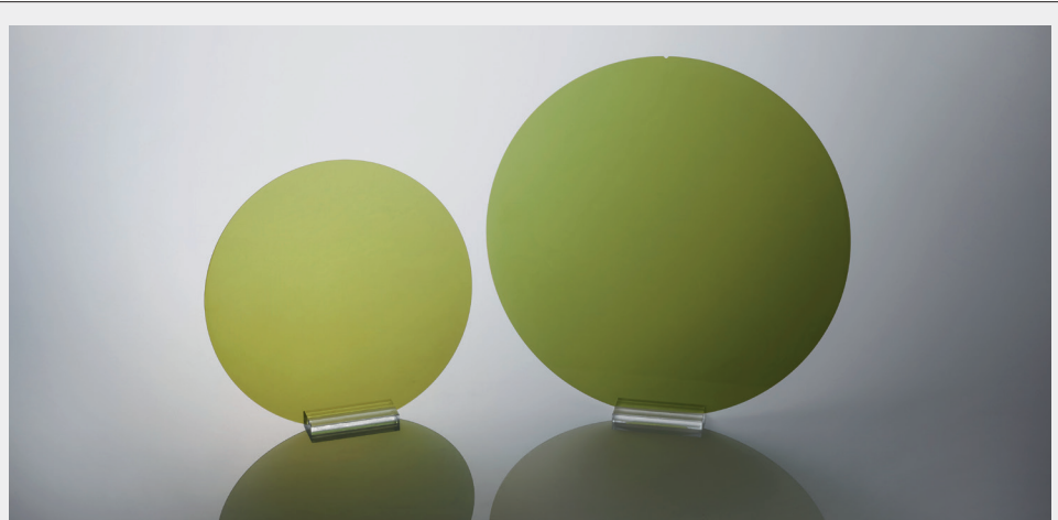
SiC epitaxial wafers (left: 150 mm, right: 200 mm). The SiC industry is transitioning toward 200 mm wafers, with the larger format providing substantially more usable surface area for semiconductor production. STMicroelectronics estimates that 200 mm wafers can deliver 1.8-1.9 times as many working chips as 150 mm wafers, helping improve manufacturing economics as volumes scale. For Homerun, this transition matters because any future entry into semiconductor-grade SiC substrates and wafers will need to align with an industry that is rapidly moving toward larger wafer formats, higher crystal quality and tighter manufacturing tolerances. (Source: Resonac )
